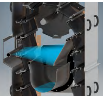
Spray bar to clean panels
