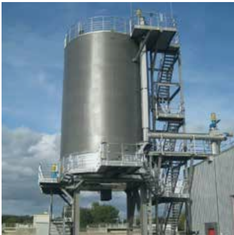
Typical two stage vertical lift sludge conveyors feeding a storage silo
