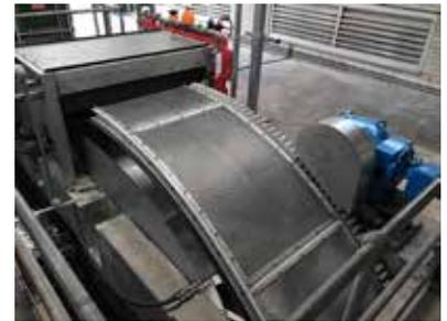
On all screens the influent is sealed from the effluent by efficient flexible neoprene rubber seals suitably shielded against mechanical damage and running on high density plastic seal flats.
