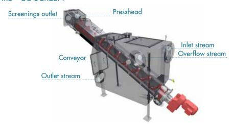
The SPIROGUARD® CC Screen is designed as a standalone unit for pump-fed applications and is available with or without a press head. Ideally suited as a tanker reception facilitator screening separation unit, it is robust and easy to install. With only one moving part, this unit is virtually maintenance free. Slow-speed combined with automatic intermittent operation ensures a reliable and efficient system.
