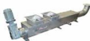
*Simple design with one moving part (double-flared inlet section shown).*
