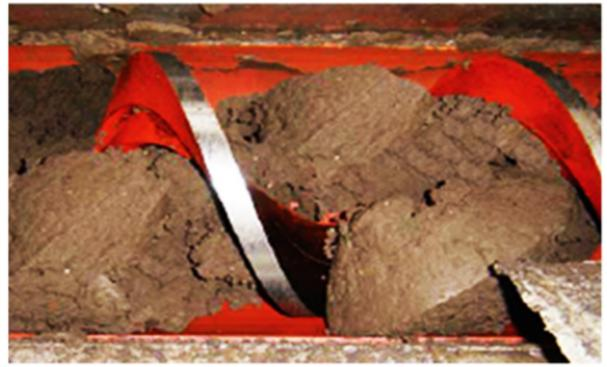
Reduced torque capability due to thin flights and higher RPM (RPM shafted  $\approx$  2-3x RPM unshafted)
